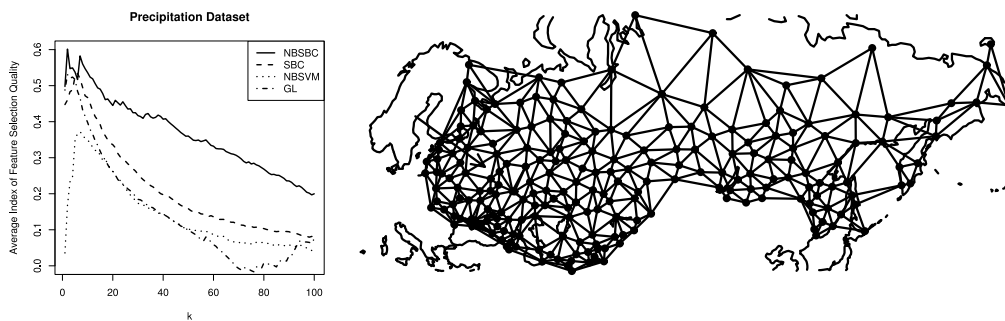
Figure 5.6: Left, average of I_{FSQ}(k) for each feature selection method in the precipitation dataset. Right, meteorological stations in the former-USSR. Each node corresponds to a different rainfall station. The arrow points to Moscow and represents the location of the target precipitation station with WMO number 27,612. The edges correspond to a Delaunay triangulation of all the precipitation stations except the target station. Links between stations that are more than 1000 km away from each other have been removed.
